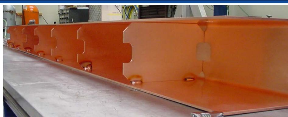
*C10100  $\frac{1}{2}$ -Hard Cu sheet bend to U-box to form a TiSP pumping plenum*
