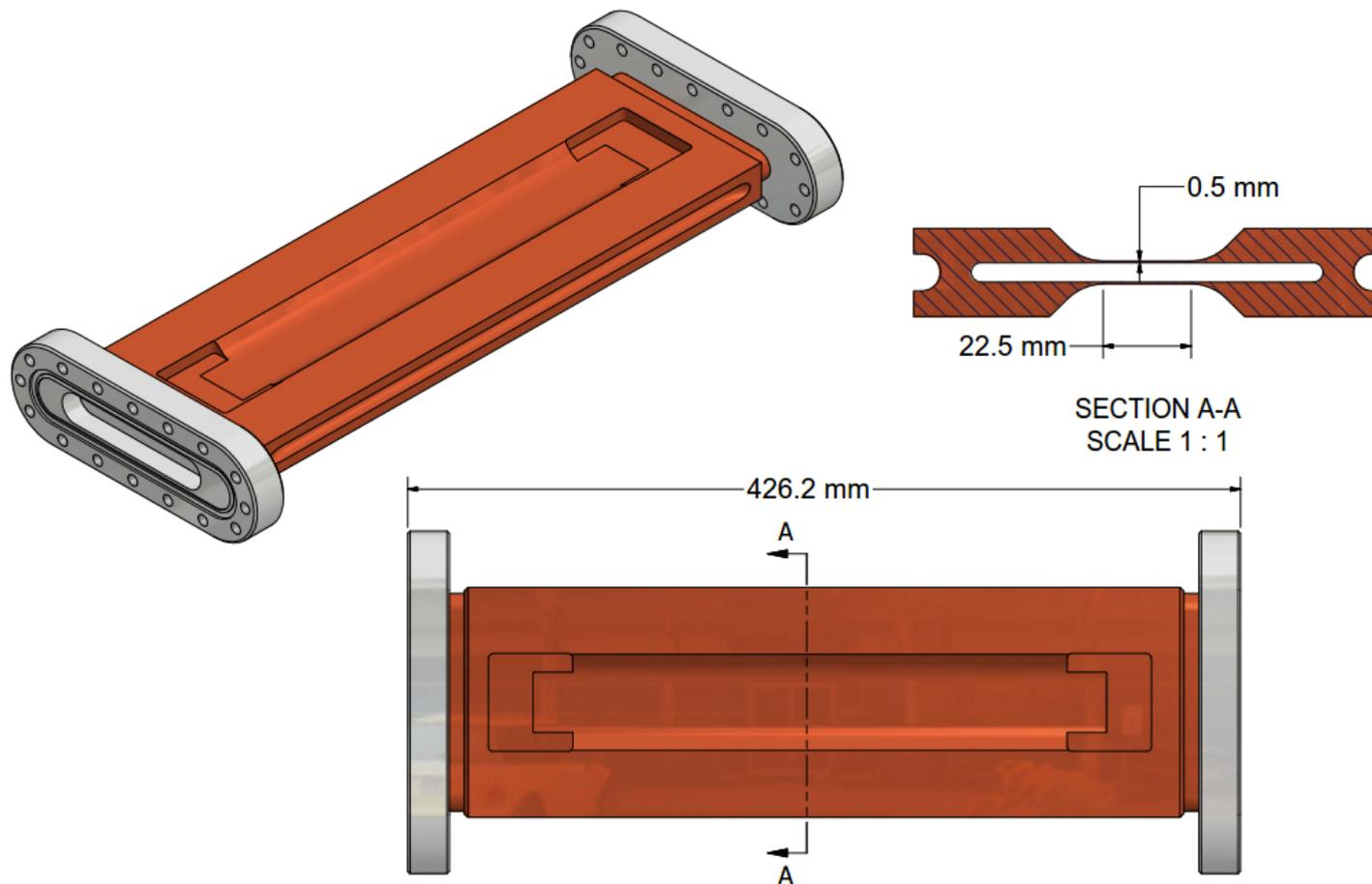
*PH Copper CuCrZr has excellent mechanical and thermal properties, thus was chosen for this thin-wall chamber. However, both Cr and Zr alloying elements may become radioactive by lost particles.*
