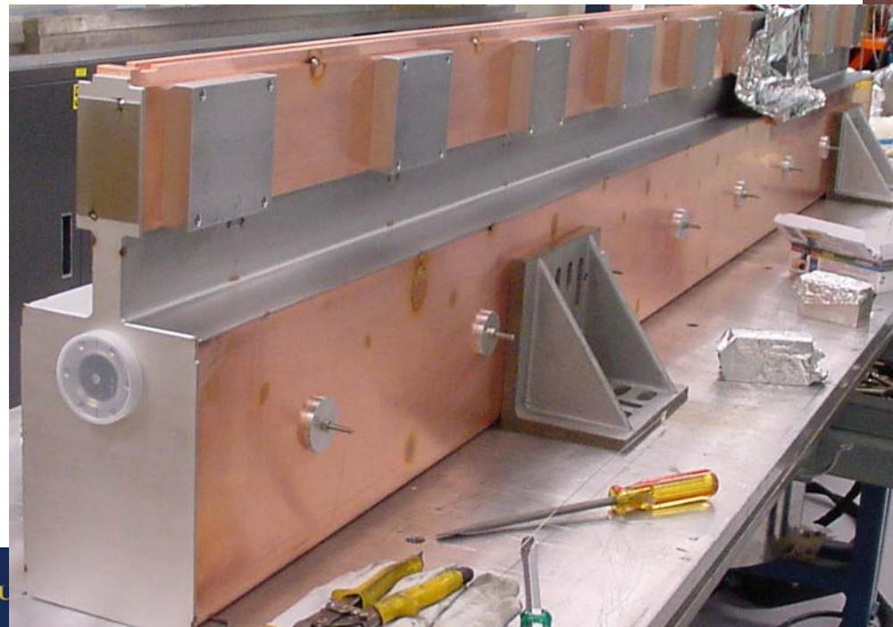
*SST L-shaped plates added to complete vacuum envelop, with enhance mechanical strength.*
