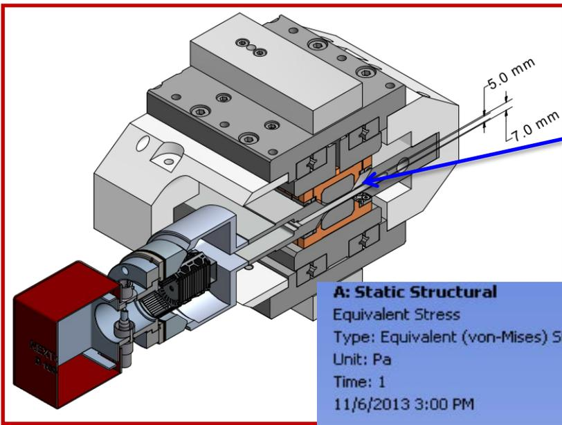
Extrusion machined to 0.6-mm thin to allow small undulator gap
